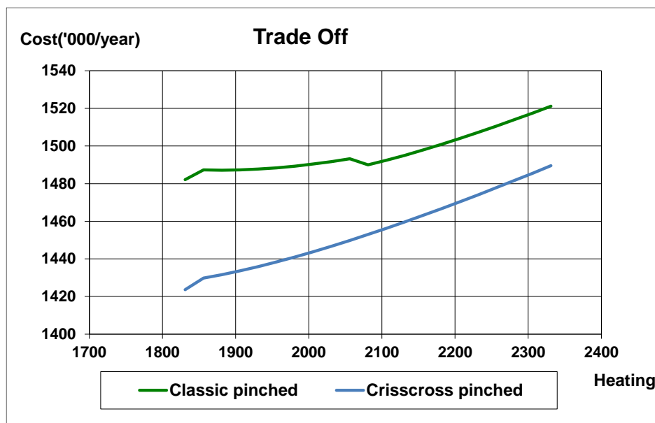
Figure 26.6 – Example 2 - Total cost as a function of heating
